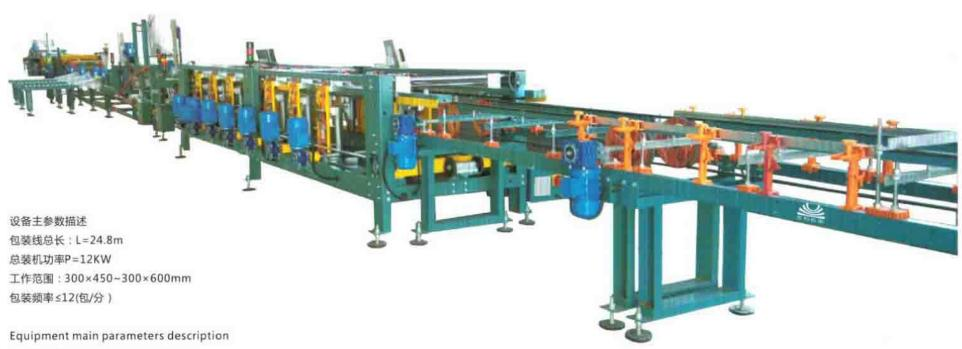
Packing line total length: L=24.8m Total installed power: P=12KW
