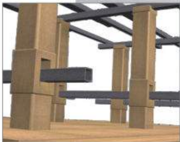
Columns, splicers and beam holders
